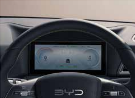
8.8" LCD INSTRUMENT CLUSTER
