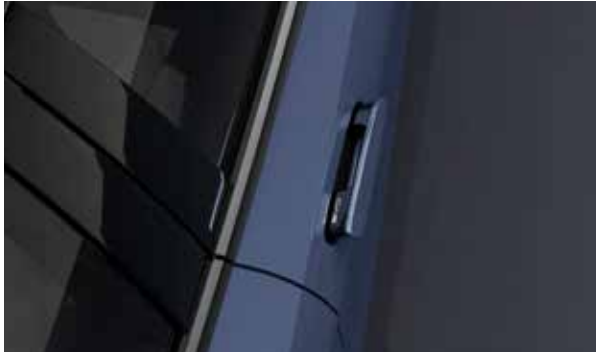
ELECTRONIC HIDDEN DOOR HANDLES Electronically retractable door handles improve the aerodynamics of the vehicle, helping in maintaining low drag coefficient
